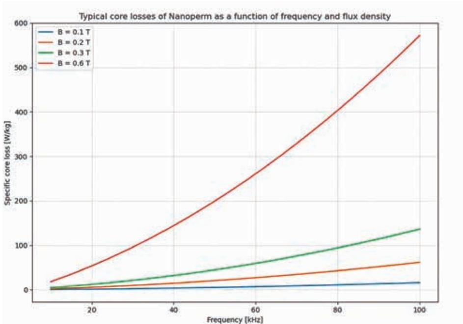
Figure 1: Example of typical core losses of Nanoperm
