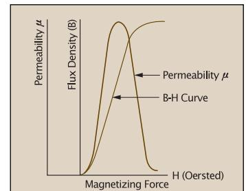
Figure 3. Variation of  $\mu$  along the Magnetization Curve
